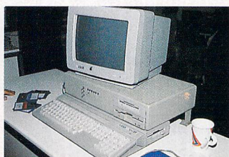
Condor's multi machine - an ST, PC and Macintosh all in one box with a hard drive and second floppy too!
